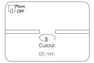
Choose the location of your new downlight, giving consideration to joists, water pipes, wiring or any other obstacles that may hamper installation. Please also ensure you have adequate ventilation and/or ceiling clearance in the relevant voids.
